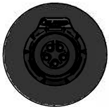
Local view B 1 : 1.5 CNLINKO-LP-5P PIN1:RS485A PIN2:RS485B
